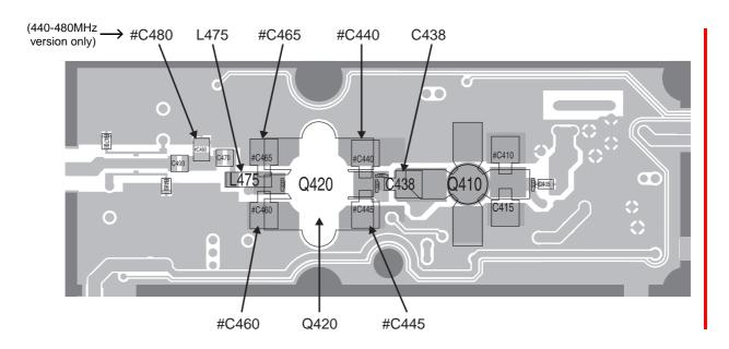
Figure 3 Components To Be Removed - Bottom Side Of PCB
