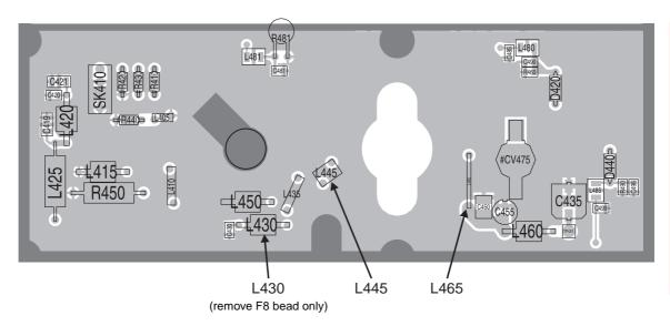
Figure 2 Components To Be Removed - Top Side Of PCB
