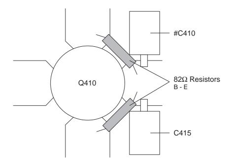
Figure 6 Placement Of  $82\Omega$  Resistors
